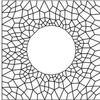
(e) Before transfinite interpolation of nodes.
