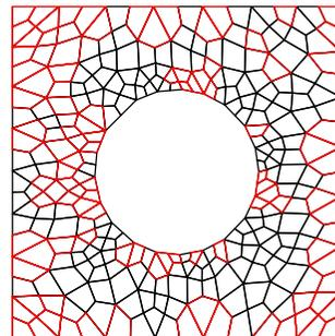
(j) Quad mesh after Tet→Quad conversion, node removal and smoothing. Bad elements detected in red.
