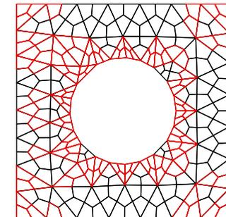
(d) Quad mesh just after Tet→Quad conversion. Bad elements detected in red.
