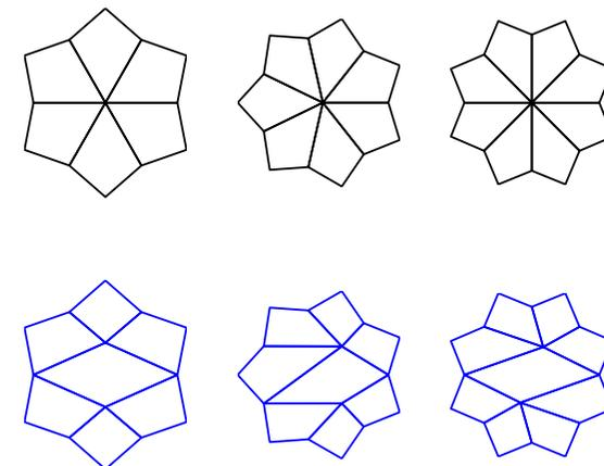
Figure: Templates for removing high valence nodes in quad meshes by inserting an element. Top row: Meshes with one high valence node. Bottom row: Meshes with high valence node removed.
