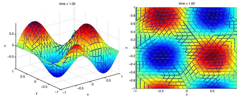
Figure: a) Snapshot of Computed solution using triangle mesh. b) Top view of computed solution. No. elements  $K = 65$  and poly. order  $N = 3$ .  $(c_x, c_y) = (1, 0.3)$ .
