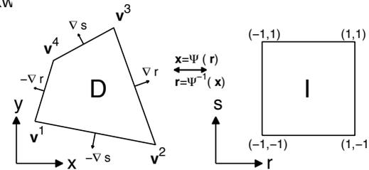
Figure: Notation for the mapping between two straight-sided quadrilaterals.
