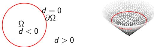
Figure: Example of a signed distance function for a circle.
