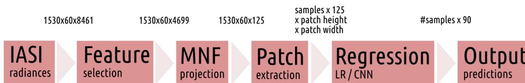
Fig. 1. Pipeline schematic: IASI spectra are first reduced from the original 8461 spectral channels by selecting a subset of 4699 channels according to noise specifications in Camps-Valls et al. (2012), which then pass through an MNF projection to reduce the dimensionality to 125 features. Subsequently, patch extraction is performed with varying sizes. Finally, either a linear regression or a CNN is used for prediction of the atmospheric profiles sampled at 90 vertical positions.
