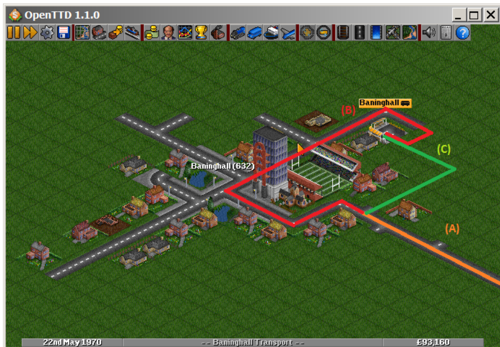
Figure 5.12: Examples of an A* algorithm result with heuristics differently prioritizing existing roads reuse. (A) The route is directed towards a town. (B) The variant is based on reuse of existing roads and minimalization of the expenses. (C) The variant is taking into account the eventual vehicle travel distance. The reader can notice that the actual distance for a traveling vehicle is longer in the case (B) then in (C).
