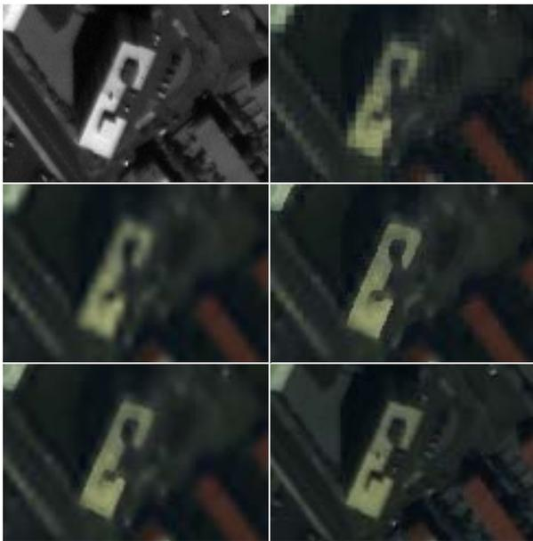
Figure 2. Results of the image fusion strategies. Another sample of the resulting images on the IKONOS data set **top left:** Input Pan-chromatic image **top right:** No smoothing. **middle left:** Uniform Weights. **bottom left:** Line Induced Weighting **bottom right:** Gradient Induced Weighting.
