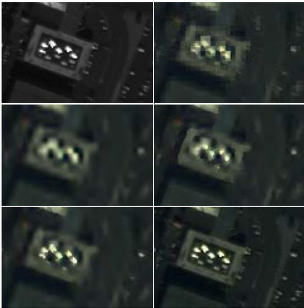
Figure 1. Results of the image fusion strategies. A sample of the resulting images on the IKONOS data set **top left:** Input Pan-chromatic image **top right:** No smoothing. **middle left:** Uniform Weights. **bottom left:** Line Induced Weighting **bottom right:** Gradient Induced Weighting.
