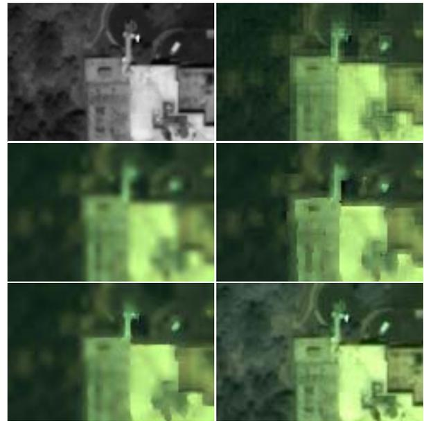
Figure 3. Results of the image fusion strategies. A sample of the resulting images on the QuickBird data set **top left:** Input Pan-chromatic image **top right:** No smoothing. **middle left:** Uniform Weights. **bottom left:** Line Induced Weighting **bottom right:** Gradient Induced Weighting.
