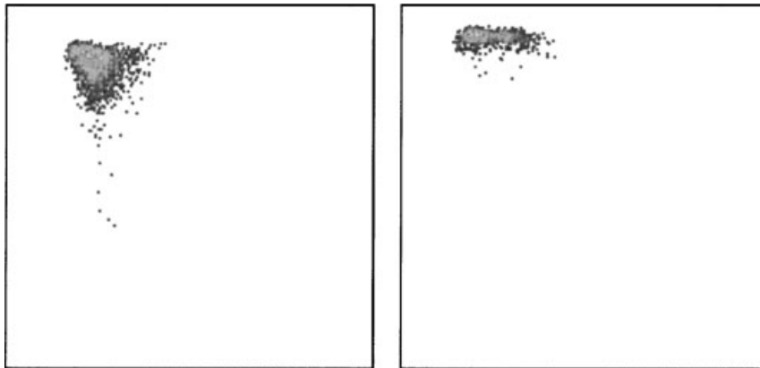
Figure 3. The left image is a 2D feature space for mussels. The right image is a 2D feature space for sand. Rows represent E1 and columns represent E2 , both in the range 0–0.5 V. Dark areas represent few observations and lighter areas represent many observations
