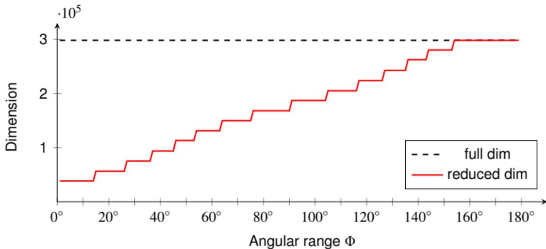
Dimensions of the reconstruction problem in the curvelet domain for an image of size  $256 \times 256$ . The plot shows the dependence of the full dimension - - - and reduced (adapted) dimension — on the available angular range  $[0, \Phi]$ .
