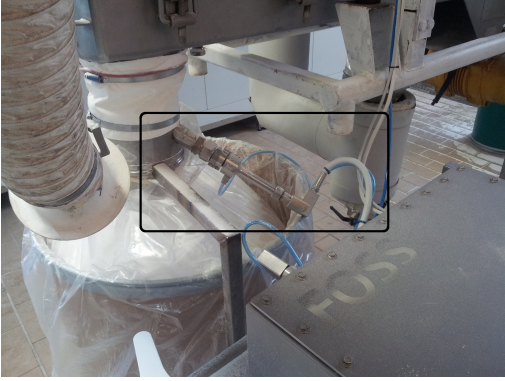
Figure 7: The VFB powder outlet with the in-line NIR analyser and the collection of produced powder.
