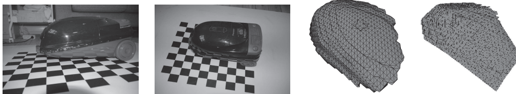
Figure 2: (left) Two images from a sequence of 25 of a vacuum cleaner. The camera flash supplied 25 normal constraints alongside the 22 point constraints. (middle) The estimated 3D shape with normal and point constraints. (right) Reconstruction with only point constraints.
