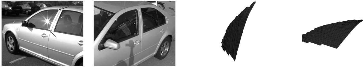
Figure 1: (left) An image from a sequence of 38 images of a car window together with the image used to find the light direction. The two point constraints available are the two sharp corners indicated with arrows. The reflectance of the sun gave 38 normal constraints. (right) The reconstructed window, which is clearly what one would expect and substantially better than what we could achieve from the two point constraints.
