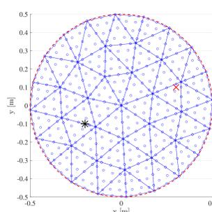
The acoustic response of the disc is simulated with and without the use of curvilinear boundary elements, in both cases using  $P = 4$  basis functions. The resulting responses are shown below.
