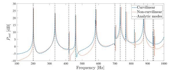
Clearly, the use of curvilinear boundary elements mitigates the apparent mistuning of the modal frequencies of the disc, which arise when the straight sided elements are used. The error is further analyzed in the figure below.
