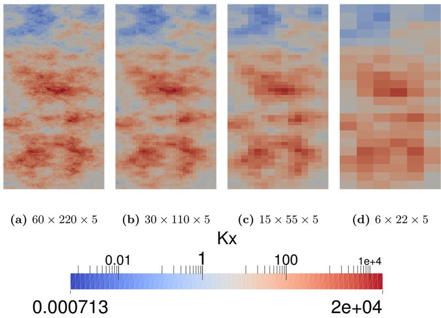
**Figure 7.1:** SPE10 top layer upscaled permeability fields using flow-based upscaling methods and fine grid permeability field. Note that for the upscaled permeability fields, only the x-component is shown here.
