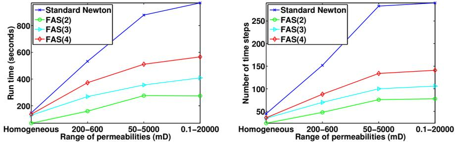
**Figure 5.5:** Left plot: Run time as a function of range of permeabilities. Right plot: Number of time steps as a function of range of permeabilities. Problem size:  $24 \times 24 \times 24$ , 5 pre- and post-smoothings, 150 days, cell sizes:  $20m \times 10m \times 2m$ .
