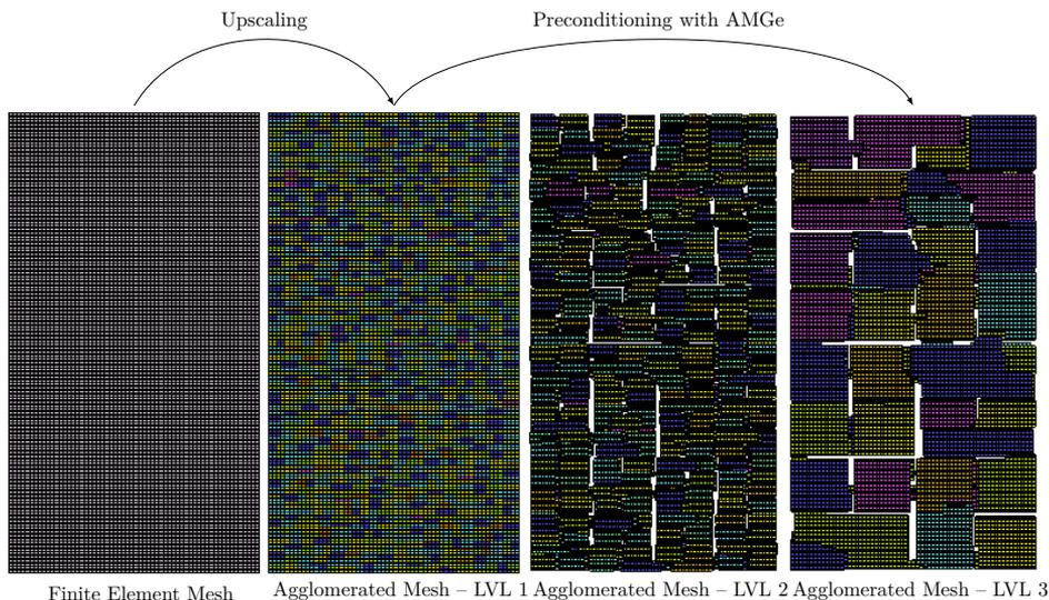
**Figure 3.9:** Full coarsening of the top 35 layers of the SPE10 benchmark case. The graph partitioner METIS is used. The agglomerated mesh at level 1 consists of roughly 32 fine grid elements per agglomerate and the agglomerated meshes at level 2 and 3 consist of roughly 16 finer grid agglomerates per agglomerate. A coloring algorithm is used to distinguish between agglomerates. Furthermore, agglomerates are slightly shrunk for visualization purposes.
