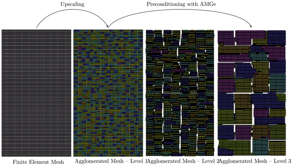
**Figure 7.4:** Full coarsening of the top 35 layers of the SPE10 benchmark case. The graph partitioner METIS is used. The agglomerated mesh at level 1 consists of roughly 32 fine grid elements per agglomerate and the agglomerated meshes at level 2 and 3 consist of roughly 16 finer grid agglomerates per agglomerate. A coloring algorithm is used to distinguish between agglomerates. Furthermore, agglomerates are slightly shrunk for visualization purposes.
