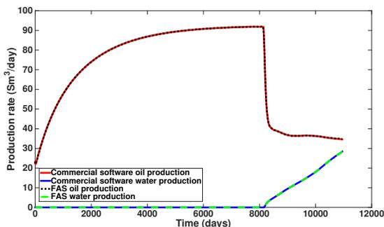
**Figure 5.7:** Quarter five-spot model validation against a commercial reservoir simulator. Grid is  $24 \times 24 \times 10$  with a domain size of 1000m x 500m x 20m. Porosity = 0.3. Permeability = 100mD. Bottom hole pressure for producer: 200 bar. Injection rate:  $100 \text{ Sm}^3/\text{day}$ .
