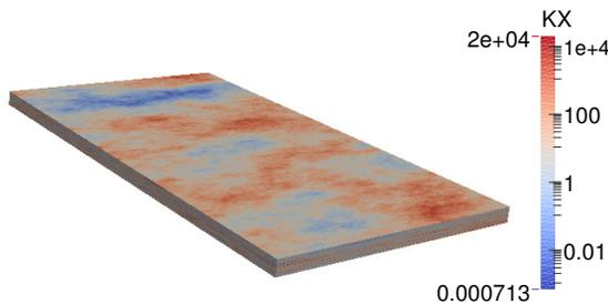
**Figure 5.11:** Top 35 layers of SPE10  $x$ -permeability field.
