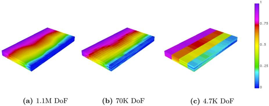
**Figure 3.2:** (a): finest grid pressure solution. (b) and (c): AMGe upscaled pressure solutions.
