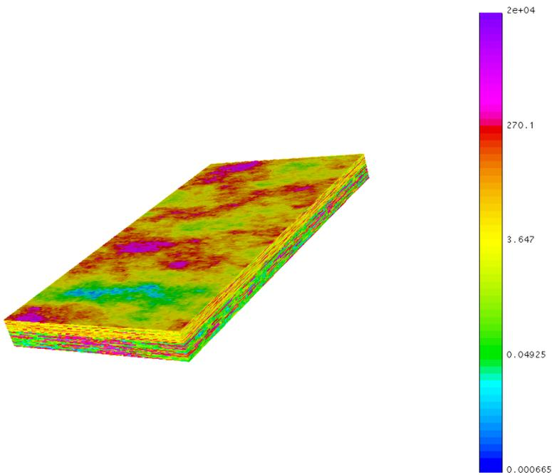
**Figure 3.1:** SPE10 permeability field in the x-direction
