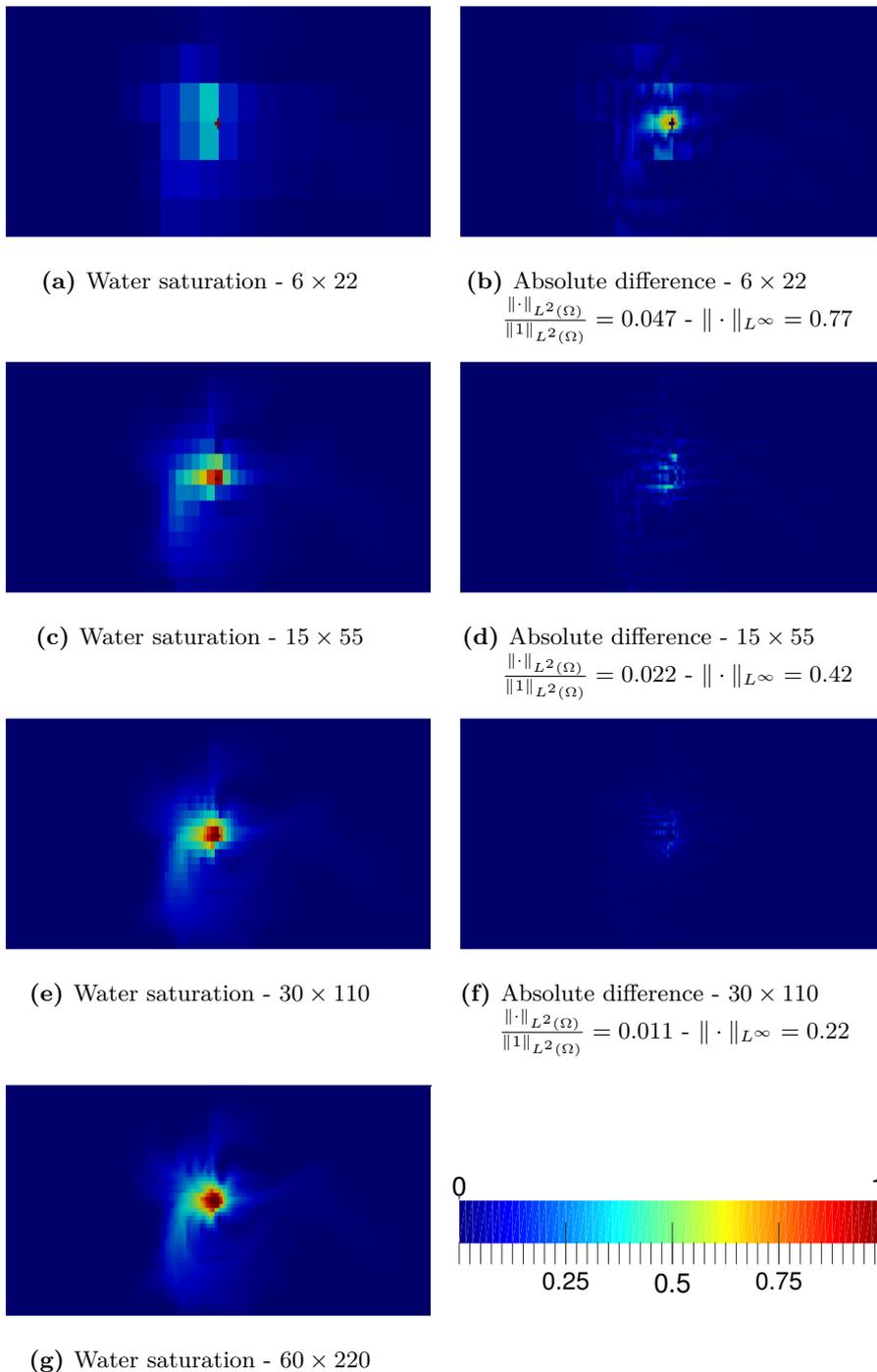
**Figure 6.7:** Left column: Water saturation after first water breakthrough (after 210 days) for fine grid reference solution and the 3 upscaled solutions. Right column: Absolute difference between fine grid reference solution and 3 upscaled solutions.
