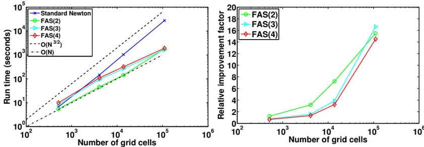
**Figure 5.3:** Left plot: Total run time as a function of the number of grid cells for SN, FAS(2), FAS(3), and FAS(4). The reservoir size is fixed at  $480\text{m} \times 240\text{m} \times 48\text{m}$ . Fixed time stepping with  $\Delta t = 1$  day. Simulation period is 100 days. Right plot: Relative improvement for FAS( $\ell$ ) over SN.
