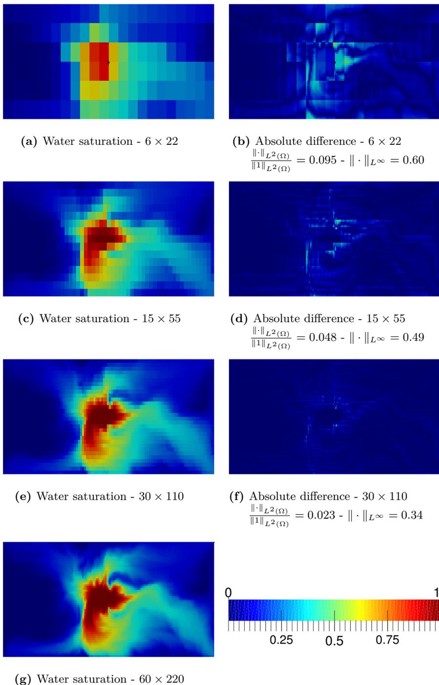
**Figure 6.8:** Left column: Water saturation after 10 years for fine grid reference solution and the 3 upscaled solutions. Right column: Absolute difference between fine grid reference solution and 3 upscaled solutions.
