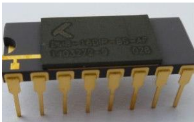
Fig. 5. The 16 DIP package containing the 8 discrete Knowm BS-AF-W memristors (source [3]).
