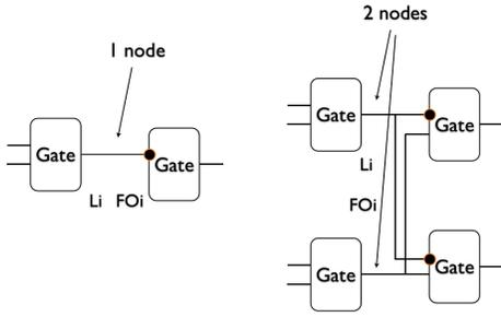
Fig. 5. Increase of node capacitances with complexity
