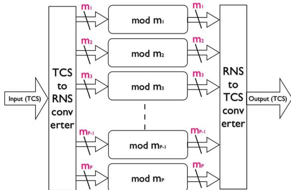
Fig. 1. Structure of RNS processor
