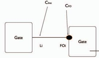
Fig. 4. Contributions to the node capacitance.
