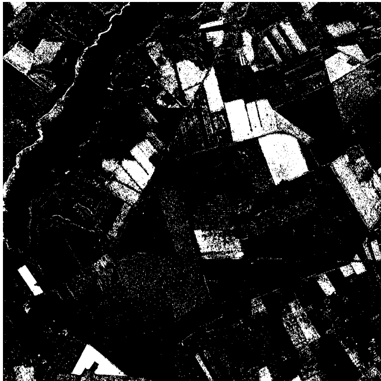
Figure 10. P\{-2\rho \ln Q \leq z\} thresholded at 0.9999 for C64/L64 vs C65/L65, full polarimetry.
