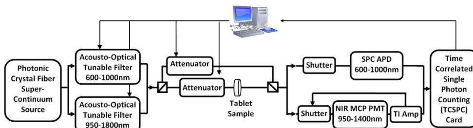
**Figure 1.** PTOF spectrometer system diagram. PCF SCS is used in combination with either AOTF to generate tunable probe pulses.
