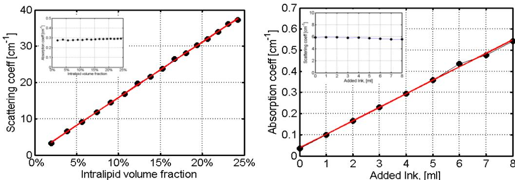
**Figure 3.** Added scatterer (left) and absorber (right) solution series. Corresponding inserts show stability of the complementary parameter i.e. absorption and scattering on the left and right respectively.
