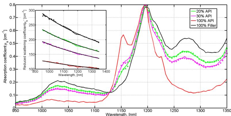
**Figure 4.** Absorption spectra of ibuprofen (red), mannitol (black) and two characteristic tablets with 20% and 30% ibuprofen content. Mixed tablet absorptions fit a linear combination of the ibuprofen and mannitol spectra, shown as open circles. Inset shows correspondent scattering spectra fitted with Mie type-dependence.
