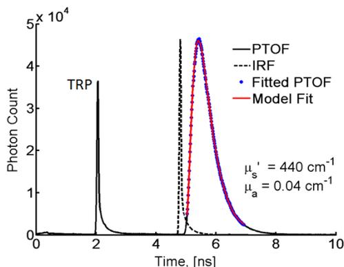
**Figure 2.** An example of the recorded PTOF distribution and IRF both having timing reference pulse (TRP) inscribed. Model fit is also shown as a red line.
