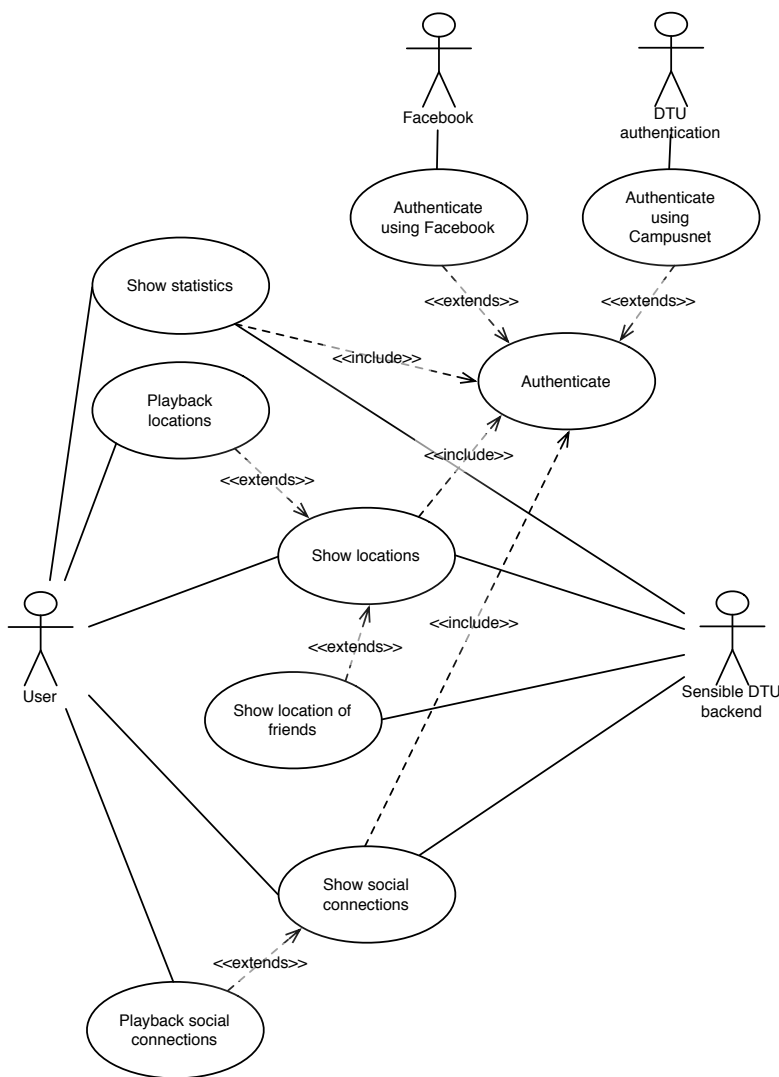
Figure 5: A use case diagram for the visualisation application.
