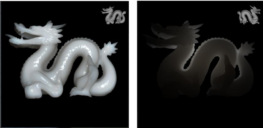
**Figure 6.6:** The Stanford Dragon 3D model rendered with the Dipole method. When the model is illuminated from behind translucency is visible, and the thin surfaces allow more light to exit.
