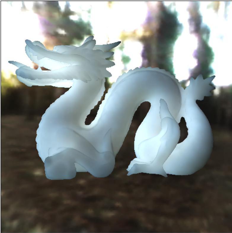
**Figure 5.26:** Translucent object rendered with diffuse illumination from the environment map. The sample points have been uniformly distributed using the point relaxation procedure described in this section. The low frequency noise is not visible anymore
