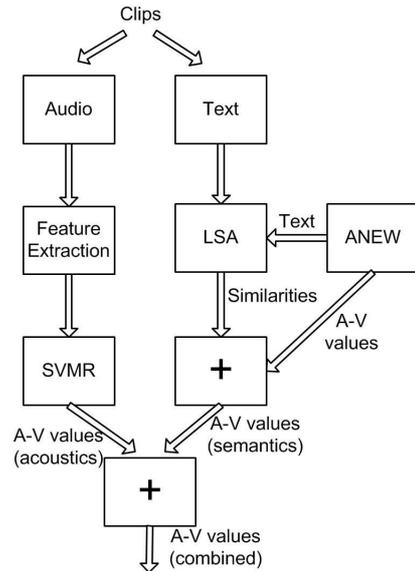
Fig. 2. An overview of the framework. The (+) sign represents that the inputs are combined, the details of the combination methods are in the relative sections.
