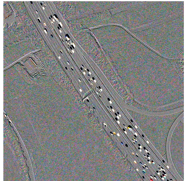
Fig. 2. Simple band-wise differences, note the noise in the no-change background.
