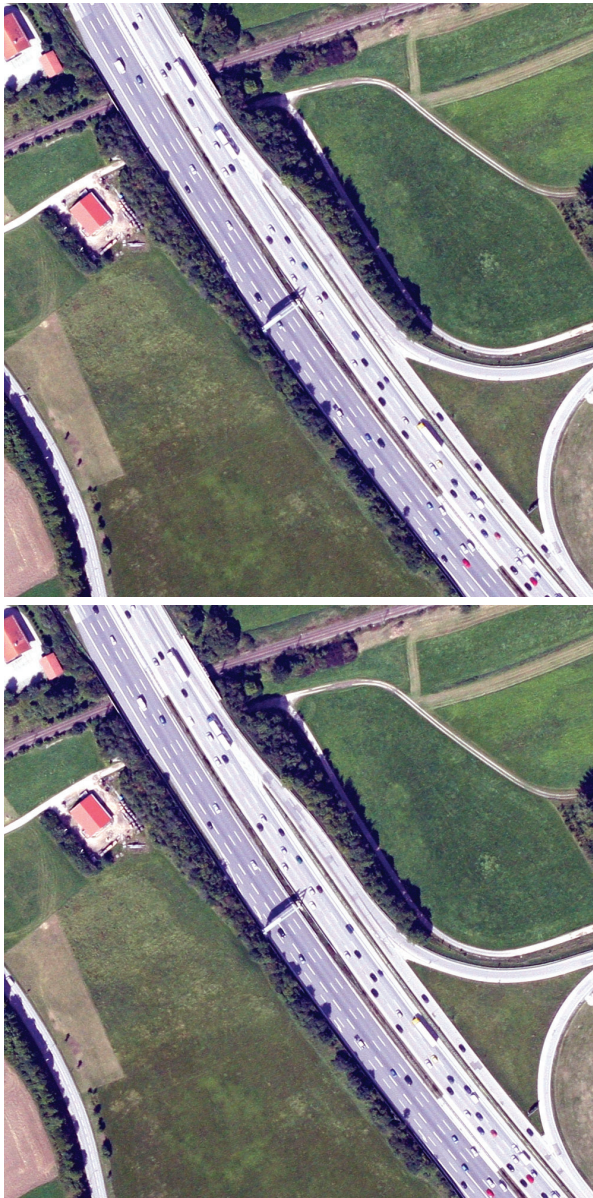
Fig. 1. DLR 3K camera system RGB images taken 0.7 seconds apart, note the moving cars on the motorway, 1000 \times 1000 pixels.
