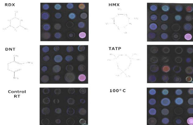
Figure 5. Difference maps of the colorimetric sensor array obtained in the presence of DNT, RDX, HMX, and TATP at elevated temperature 100 °C. Images were generated after the mathematical calculations of the color changes; and presented as the difference map obtained from the absolute values of RGB values of each dye spot before and after the exposure of targets.
