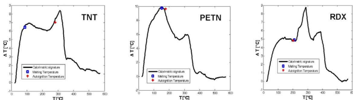
Figure 3: Calorimetric signature of respectively TNT, RDX and PETN. The melting temperature and the auto-ignition temperature is shown on the graph.
