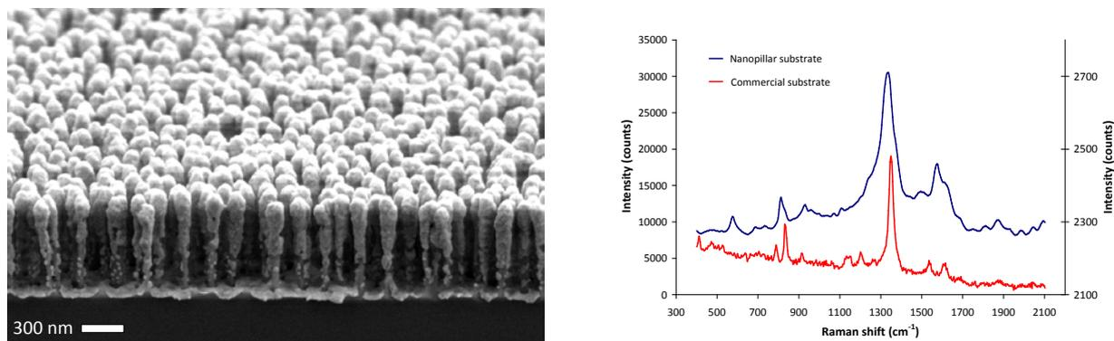
Figure 4: Left: Scanning electron microscope image of nanostructured silicon surface optimized for enhancing the Raman effect. The silicon surfaces are coated with thin film layers of silver / gold. Note the large surface area. Right: Raman spectra (785 nm excitation, 1s acquisition) of DNT evaporated onto the nanopillars substrate with a commercial substrate inserted as a comparison. The nanopillars substrate has a two orders of magnitude stronger signal. Note the two different y-axis.
