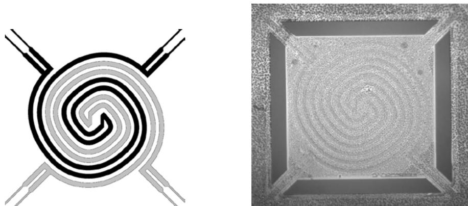
Figure 2: left: The silicon resistors are designed as two spirals inside each other with small vias to the connecting substrate. The small vias dissipate extra heat at the suspensions to the substrate compensating for diffusion losses. The spiral dissipates heat evenly across the membrane for a uniform temperature distribution. Right: Optical microscope picture of a membrane covered with 48 ng of TNT.
