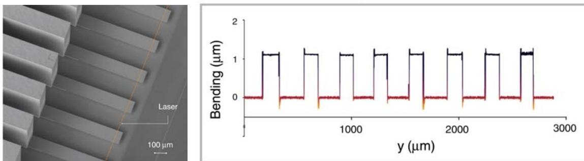
Figure 1: Left: SEM picture of the Au coated silicon cantilever array. Right: Single chip profile, consisting of around 1000 points for each of the eight cantilevers.
