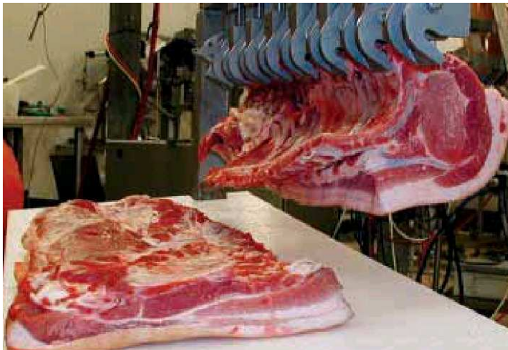
Figure 1.2: The middle cutting machine in action. The belly is on the table. The back with the ribs is hanging from the hooks.
