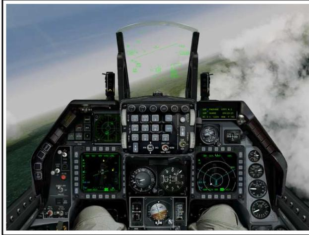
Figure 2.10: The cockpit of an F-16 fighter aircraft. Above the knees of the pilot two MFDs can be seen. The azimuth indicator is positioned to the top left, above the left MFD. (Screenshot from the Falcon 4.0 flight simulator from Microprose.)
