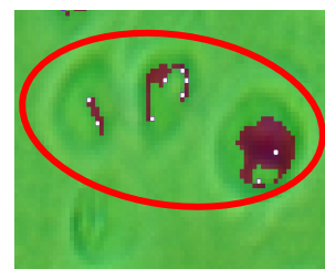
Figure 15-6: Specimen 216-11. Vague chondrocyte leads to several chondrocyte centers, illustrated (a) before and (b) after segmentation.
