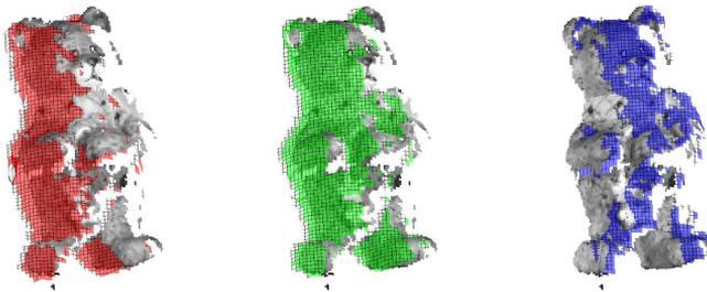
Figure 10.3: The three stages of estimating the coarse alignment of the target shape (coloured) w.r.t. the reference shape (textured): The previous global transformation (red). The previous local transformation (green). Translation to match the centroids (blue).
