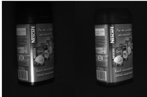
Figure 3.4: A specular surfaced object, captured under direct (left) and diffuse (right) illumination.
