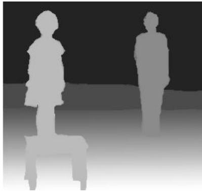
Figure 1.2: The depth map of the scene from Figure 1.1 (brighter is closer and darker is further away) (From [41]).
