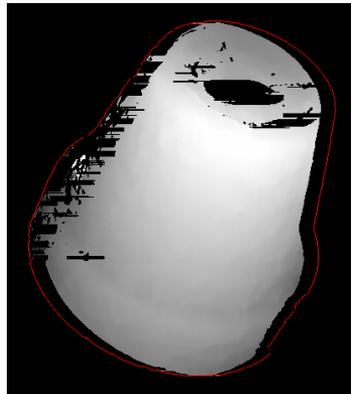
Figure 8.18: The resulting disparity map, where regions inside the object border (red) has been reduced.
