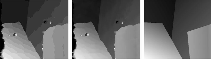
Figure 8.12: Three disparity maps of the Venus data. Pixel level based (left), sub-pixel accuracy (middle) and the true disparity map (right).
