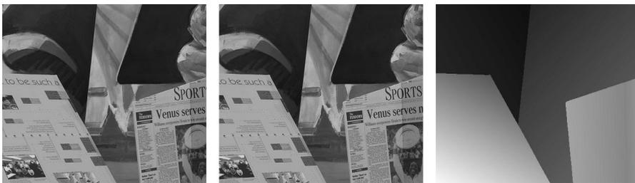
Figure 8.2: The Venus stereo pair (left and middle) and the sub-pixel accuracy ground truth disparity map of the left image.
