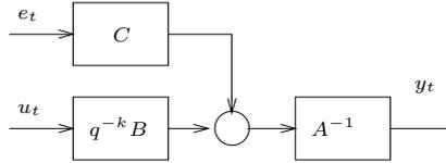
Figure 1. Stochastic system in the ARMAX form
