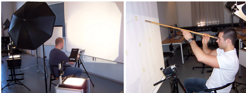
Figure 17.1: Video recording setup. ( Left ) The person recorded is indirectly illuminated. ( Right ) The gaze direction is turned at a collection of markers placed at some controlled points in 3D space. The DV-Cam is positioned in front of the person.
