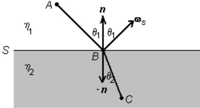
Figure 3.4: The path of light when it travels from one homogenous medium to another.
