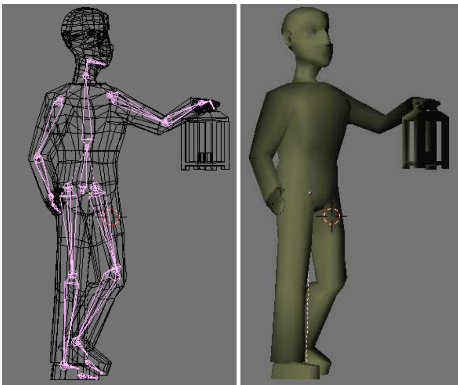
Figure 9.2: Armature of the male character in the cave scene. Notice how the mesh follows the bones.
