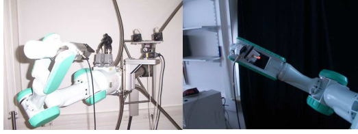
Fig. 1. Robot arm and calibration target, which were used to record the data items.
