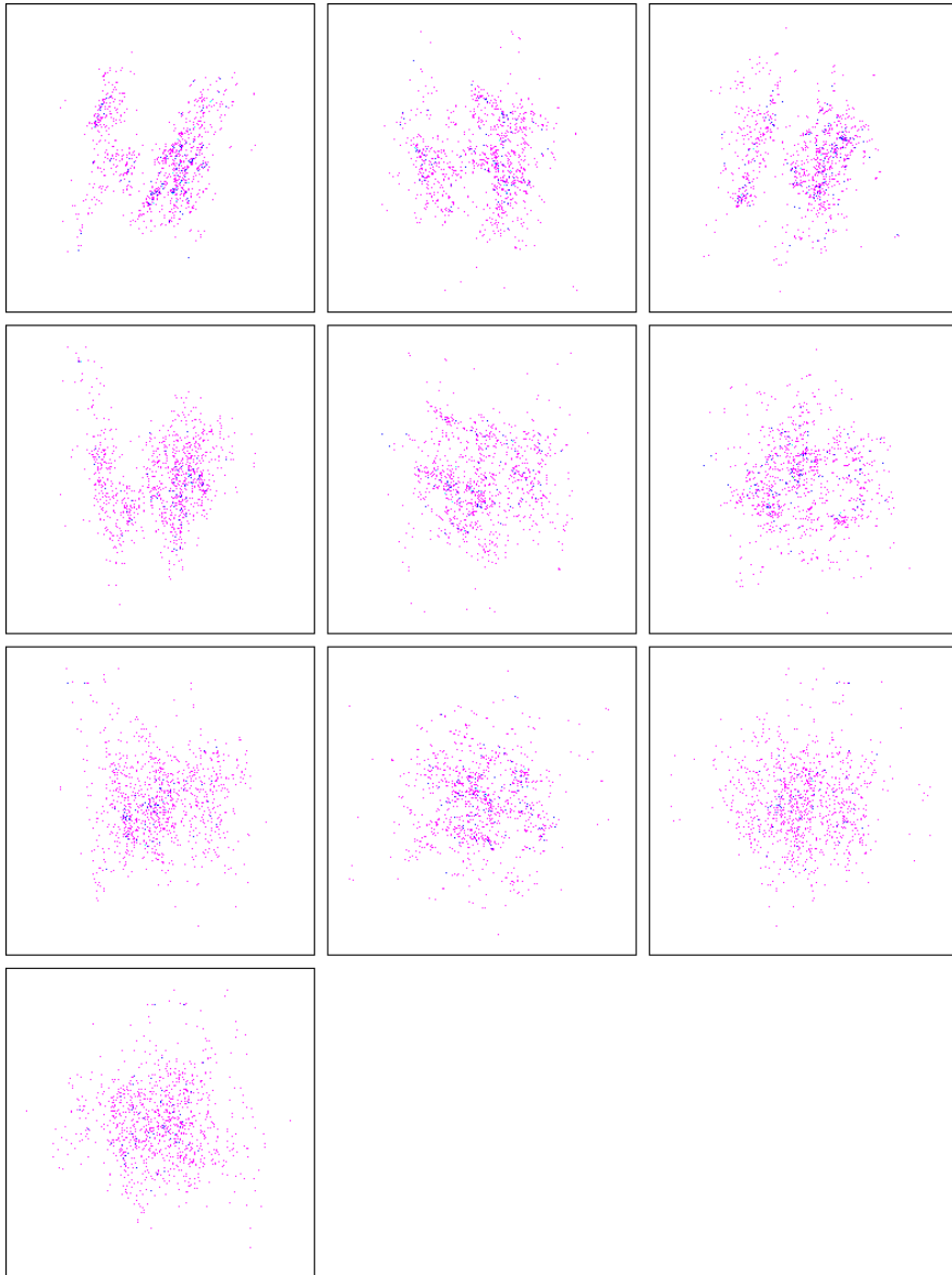
Figure 9.8: Scatter-Plots of variables transformed into the principal component space. The variables are restored geometrically rectified C- and L-band polarized EMISAR amplitude data from the three test sites at Trehøje, Benlighøj and Stenhøje at Mols Bjerge 3 and 4 June 1997, see text page 216. Starting in the upper left corner going right the scatter-plots are: PC1/PC2, PC1/PC3, ..., PC4/PC5. The colours magenta-blue-cyan-green-yellow and red represent the number of hidden observations 0, 1, 2, 3, 4 and > 4
