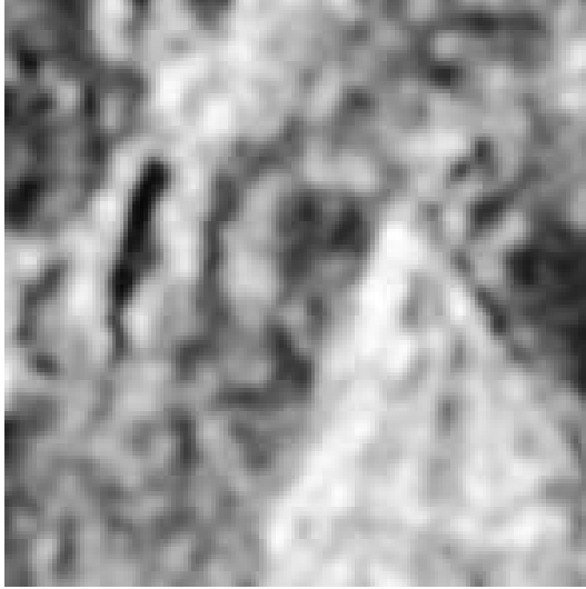
Figure 5.11: The restored C-band VV-polarized EMISAR data in Figure 5.2 after 9 iterations using the exponential prior and ICM with the optimized parameters \alpha = 2 and \beta = 5 . The data are histogram equalized using the beta distribution with the parameters 3 and 2.
