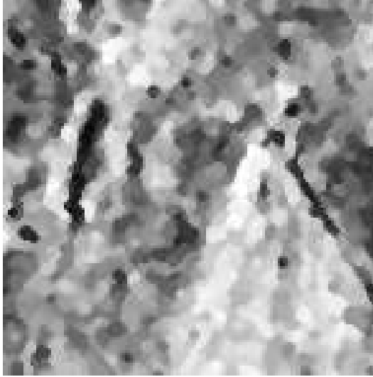
Figure 5.27: The restored C-band VV-polarized EMISAR data in Figure 5.2 after 9 iterations using the Gamma pixel prior and ICM with the optimized parameters \alpha = 2 , \beta = 0.5 and k = 5 . The data are histogram equalized using the beta distribution with the parameters 3 and 2.
