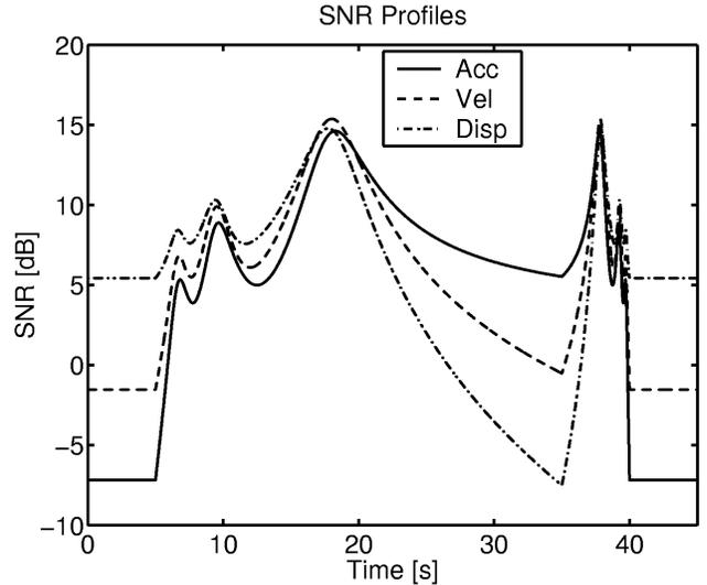
**Fig. 3.** Variation in SNR. This figure shows the non-stationary behaviour of the signal to noise ratio when the fundamental frequency and harmonic orders changes as shown in figure 2. The noise variance is set for each of the three responses, such that an overall SNR of 10 dB is achieved.
