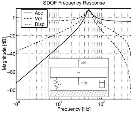
**Fig. 1.** Frequency responses for the second order filter simulating the mechanical system with a single degree of freedom (insert): Acc - acceleration responses; Vel - velocity response and Disp - displacement response.
