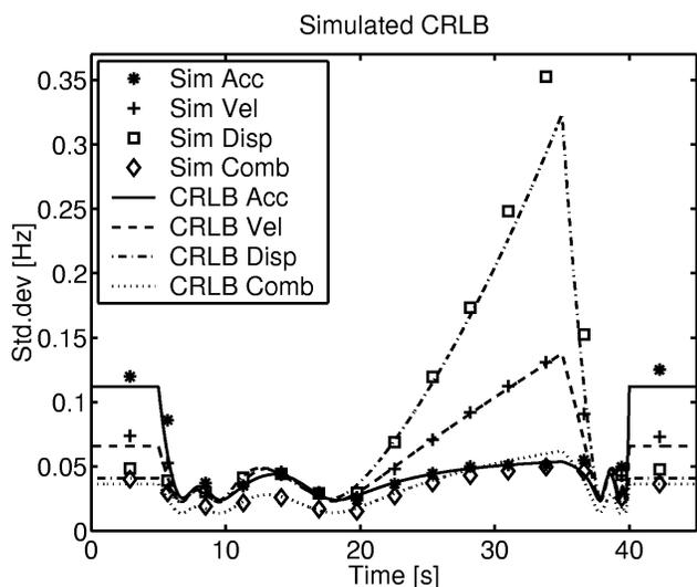
**Fig. 4.** Cramér Rao Lower Bounds. The estimated standard deviation,  $\sigma$ , of 100 Monte Carlo simulations of tracking fundamental frequency in the three different response signals are plotted here using symbols. With lines are shown the theoretical limits computed according to [4]. There is strong agreement between simulations and theory. It is noted that tracking on the joined posterior improves the estimate significantly.
