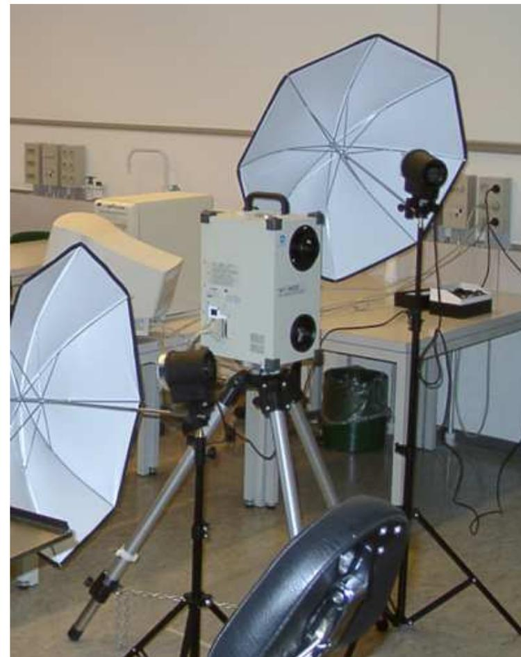
Figure 4.1: The scanning setup. The lens can be seen on the upper front part of the camera. The opening below holds the laser.
