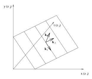
Figure 2: k is the unit normal vector of the iso-grey level planes generated by a translating line.  $k_1$  is the unit direction vector of the translating lines, and is therefore perpendicular to k.  $k_2$  is a vector perpendicular to k as well as  $k_1$ . The normal flow is found as the projection onto the  $(z_1, z_2)$  of  $k_2$  multiplied so its temporal coordinate equals 1.
