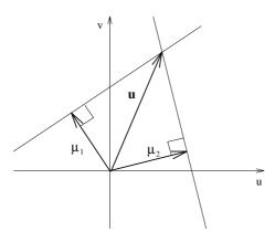
Figure 3: The true flow, u, is constrained by the linear constraints given by the two normal flows,  $\mu_1$ , and  $\mu_2$ .
