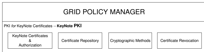
Figure 8.3: Components of a Grid Security System
