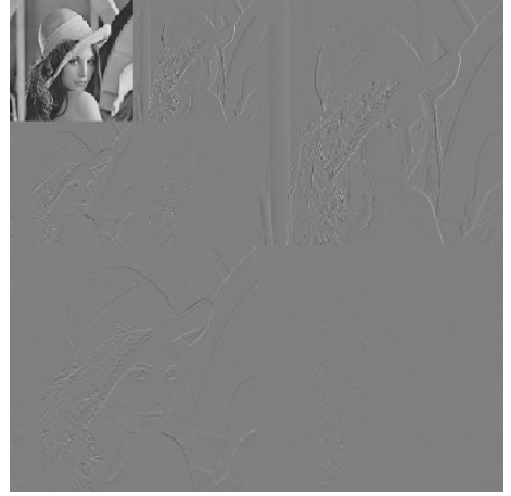
Fig. 1. The wavelet coefficients of a two-level octave decomposition using the Haar wavelet.
