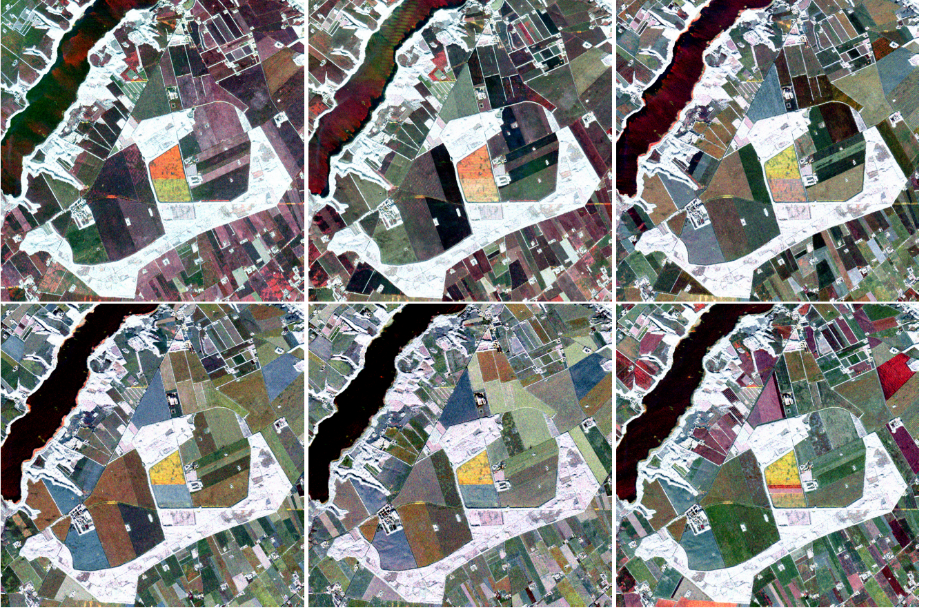
Fig. 1. EMISAR L-band monthly data March-August covering an agricultural region near Foulum, Denmark, logarithms of eigenvalues as RGB ( \ln \lambda_1 is red, \ln \lambda_2 \leq \ln \lambda_1 is green, and \ln \lambda_3 \leq \ln \lambda_2 is blue; same stretch to all \ln \lambda_1 , same (but different) stretch to all \ln \lambda_2 , etc.
