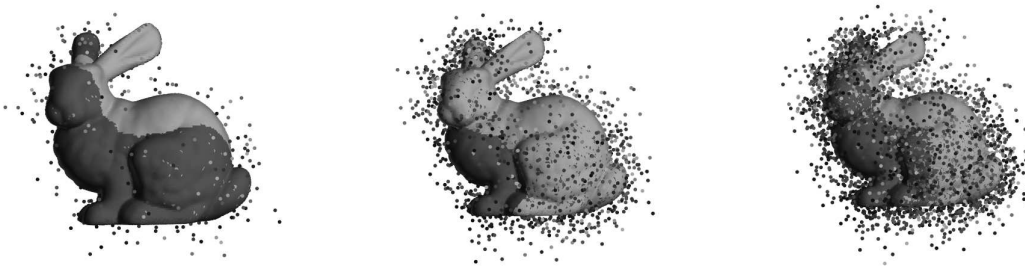
Figure 4.2: Registration of the bunny with outliers added. The amount of outliers in each example is 1%, 5% and 10%. It is clear to see the registration is working for the two first but the amount of outliers make it hard to see the bunny in the last.
