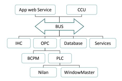
The non-physical devices connected to the bus are the database, the CCU and the AppService. Although these subsystems are out of the scope of this report there are subjects specific to these integrations that have changed the way a part of the system works. In addition to that the choices of how these systems are connected have relevance.
