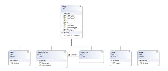
This model show the top of the system and it is used to relate sensors and actuators to a subsystem. In the message space a subsystem is a part of the *StateResponse* message that describes the current state of a subsystem. The distribution of state will be described when the data model and message space has been described in detail.
