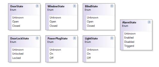
These enumerations show the suggested valid states of the actuators of the system. The unknown option was implemented as a valid null value and it can be interpreted by the individual subsystem as they wish.
