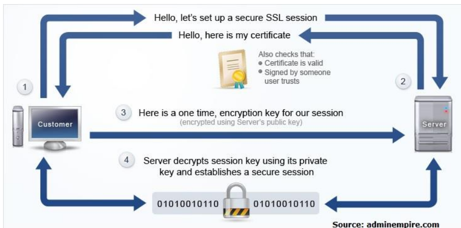
Figure 35: SSL setup between browser and server software [20]
