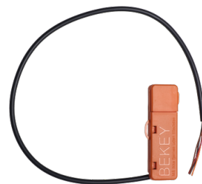
Figure 3.2: The BeKey that hooks into existing electronic unlocking systems.[9]
