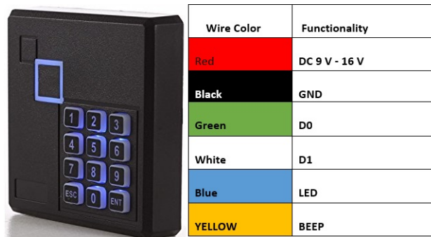
Figure 4.9: Reader along with the Wire Connection Chart
