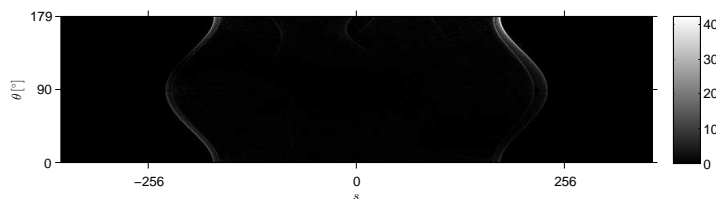
Figure 6.7: Absolute difference in two sinograms using MATLABs radon() and A in (6.8).
