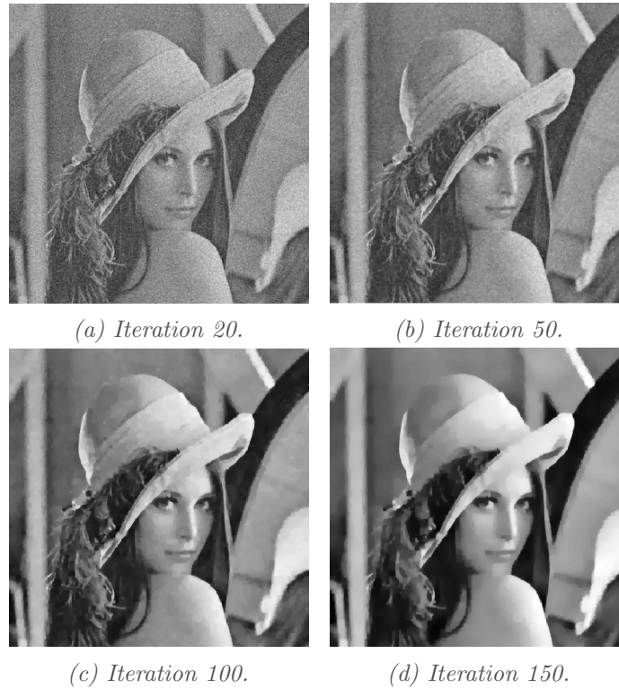
Fig. 7.7: Denoising 2D: Total variation reconstructions at different times with \Delta t = 1/2\Delta x .
