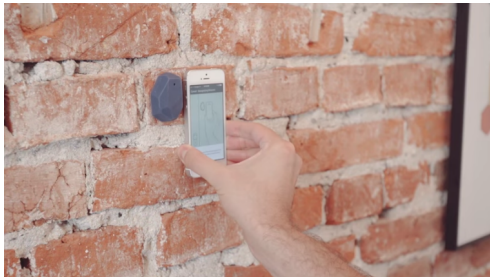
Figure 30: The configuration starts by placing a mobile device next to one of the beacons in the area to confirm the location.
