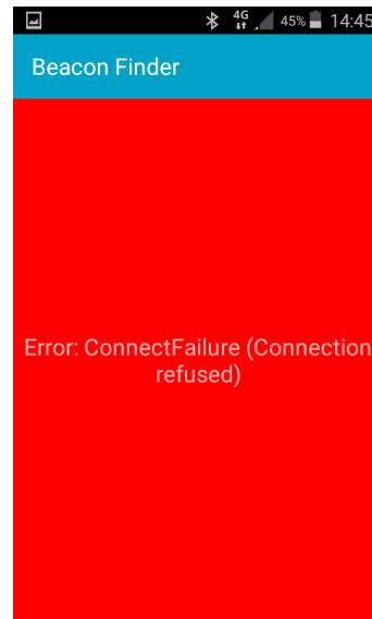
(d) When the system get an error on client-side, it is displayed on a red screen with the error. In this case the connection is lost to the server(REST web-service).
