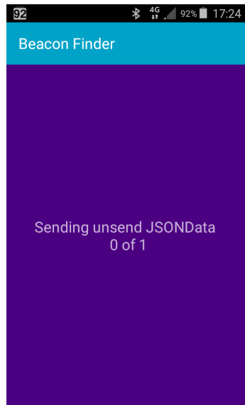
(c) Screen display when there are unsend beacon-data and the application is trying to re-send them to the REST web-service for storage. Screen text saying "Sending unsend JSONData 0 of 1".
