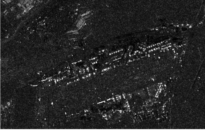
Fig. 2. -2 \ln Q omnibus change detector for Sentinel-1 C-band VV/VH dual polarization data, diagonal only, over seven time points from 10 Feb 2016 through 12 Nov 2016, stretched linearly between 0 and 100 .
