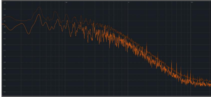
Figure 8.1: Spectrum of the implemented low-pass filter effect for a white noise input signal with constant gain all over the spectrum, showing the decay of frequencies above the cut-off frequency.
