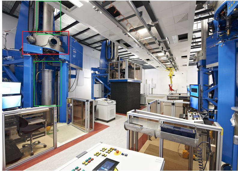
Figure 1.1: Image of the production hall at Topsil GlobalWafers A/S. To the left is shown a float zone machine in an open position. In the green boxes are the crystal holders that contains and pulls the silicon. In the red box is the pressurised chamber. When used in production, the two holders locked into the chamber and sealed.
