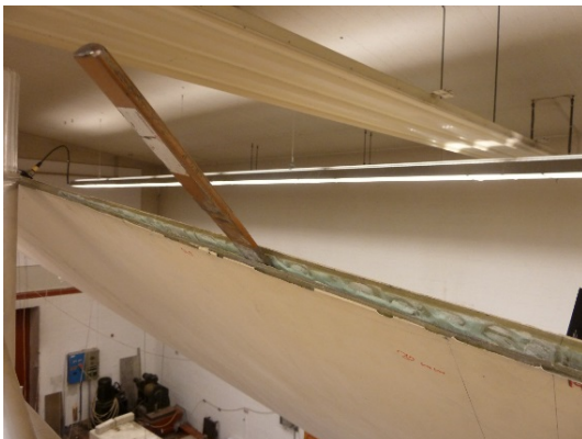
Figure 5. Blade damage in the trailing edge, with the chisel used to introduce the damage
