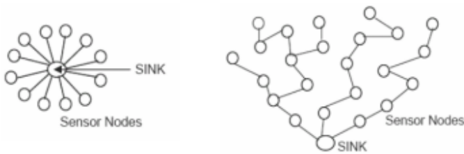
Figure 2.3: Single-hop and multi-hop topologies in WSNs [2]
