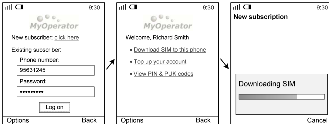
Figure 4.9: Concept: pages served from an operator’s subscription server. Left: the first page allows new subscribers to register, or existing subscribers to log in. Middle: example of what a welcome page for an existing subscriber could look like. Right: a VSIM is downloaded from the subscription server to the terminal. Source: own work.
