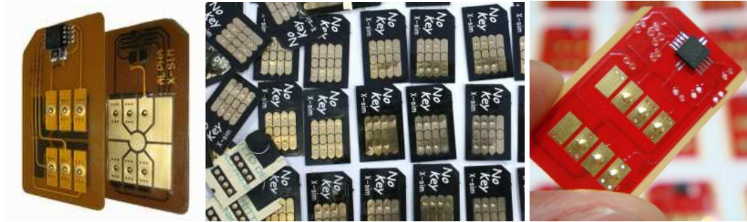
Figure 5.3: Examples of commercial SIM-Lock bypassing devices designed to fool the terminal into thinking the SIM has a valid IMSI. These ‘X-SIM’ devices are placed between the SIM card and the terminal’s SIM connector intercepting and altering the communications. Source: internet bulletin board (GSM Forum).
