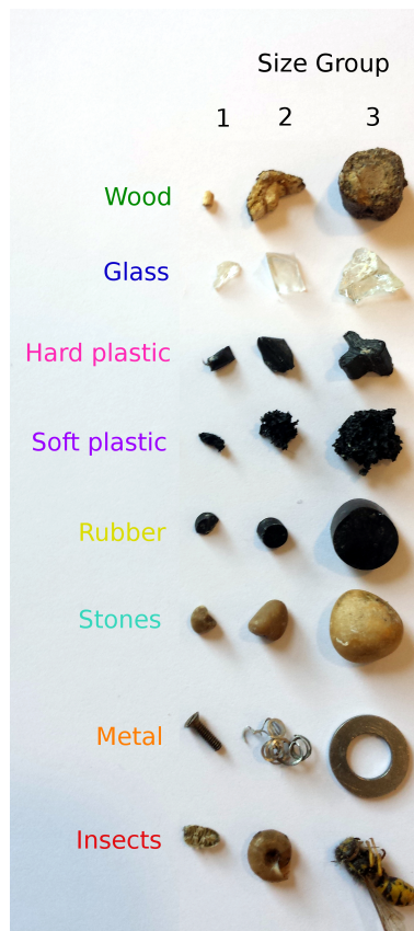
Figure 2.7: Selected foreign bodies, with approximate sizes of 2x2x2, 3x3x3 and 4x4x4 mm, from left to right.
