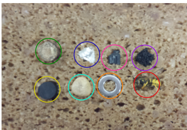
Figure 1.2: Purple: Soft plastic, Pink: Hard plastic, Blue: Glass, Green: Wood, Red: Insect, Orange: Metal, Cyan: Stone and Yellow: Rubber.
