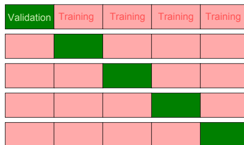
Figure 2.6: An example of 5-fold cross-validation. The complete data is split into five equally sized subsets. Four of the subsets (red) are used as training, while the last subset (green) is used for validation. This is done five times, such that all five subsets are eventually used as validation set. The mean value of the individual accuracy estimates, is the cross-validation estimate of the accuracy.
